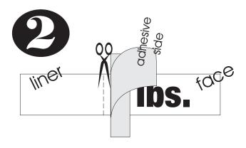
Fold left half of decal over, peel face from liner of decal and cut off liner (if not slit). If slit be sure the tape is near but not over the slit. Fan decal back and peel off one side of the liner.
