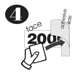
Remove masking tape and fold opposite half of decal over and discard liner. Squeegee this side down, in the same manner.
