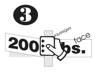
While holding the peeled side slightly away from the surface squeegee the left half down to substrate using soft, then harder strokes from center out. Care should be taken to not trap air bubbles. The adhesive will grab immediately.
