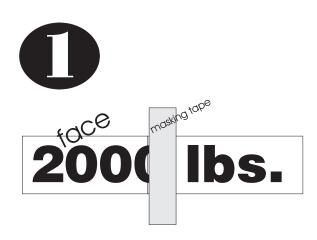
Position decal at proper location and apply vertical "hinge" of masking tape.
